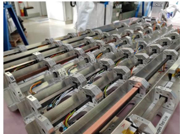
Figure 7. Sample target stations of Multimat-2 experiment.
