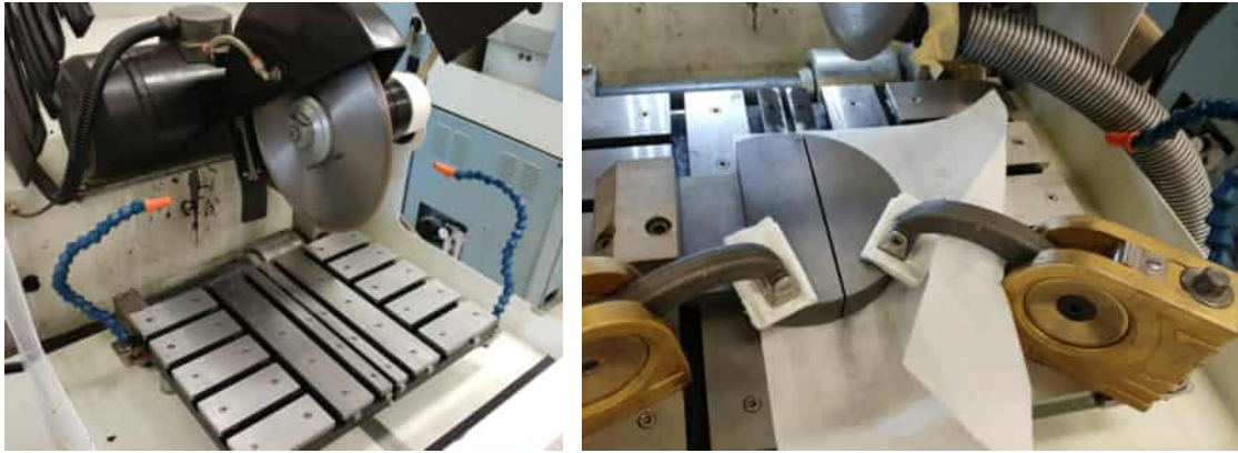
Figure 4.36: Slicing process with circular saw, diamond disk ( \text{Ø}254 \times 1 \text{ mm} ) The conventional SiC disk work also well, but having larger thickness they produce more graphite dust and waste more material.
