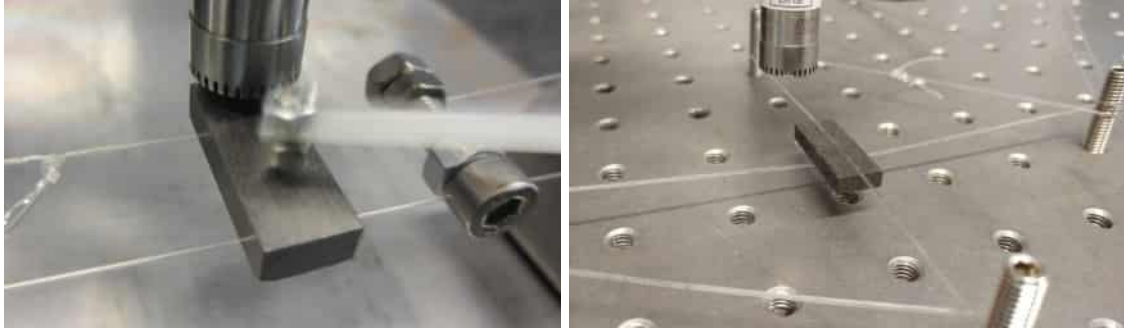
Figure 3.7: IET experimental set-up. Nylon-wire supports for exciting the flexural (left) and torsional (right) frequencies. Left picture shows the specimen being impacted with the excitor. Specimens shown are 25 mm long.
