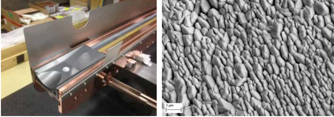
Figure 1.27: (Left) TCSPM collimator prototype before installation in the LHC. The jaw is made of MoGr absorber blocks coated with a strip of Mo and another of TiN for testing purposes. (Right) SEM observation of the surface of Mo film (7 \mu\text{m} ) deposited at CERN on MoGr MG-6403Fc.
