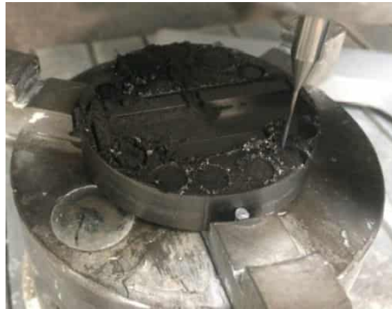
Figure 4.35: Milling specimens from a sintered plate
