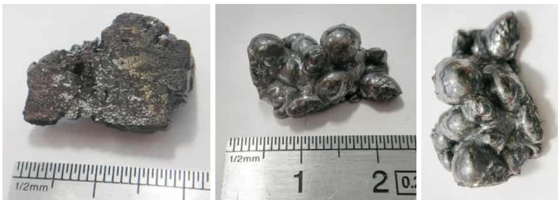
Figure 6.29: Cr-C LP spill material from CG-1100B0 plate. One surface was polished to reveal its internal structure, which shows visible grown graphite flakes (left).
