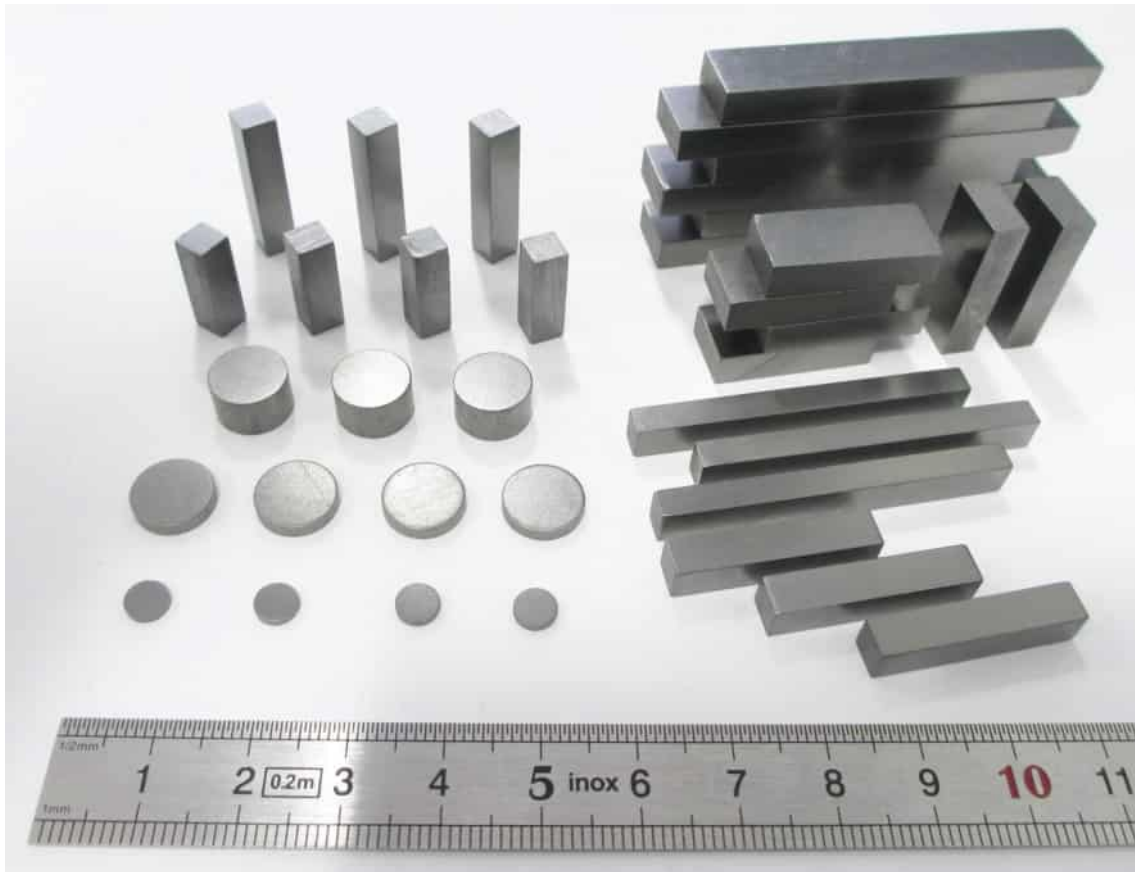
Figure 5.40: CG-1100Ba specimens for characterisation machined by Brevetti Bizz.
