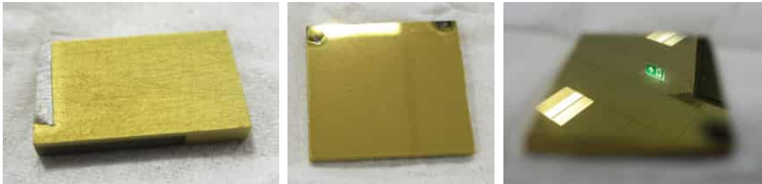
Figure 1.26: Coating tests of TiN ( 5\mu\text{m} ) on (left) MoGr MG-6530Aa ( 10\times 15\text{ mm} ), and (centre/right) glass ( 25\times 25\text{ mm} ). Note how the substrate roughness defines that of the coating; the smooth surface of glass produces a perfect TiN mirror that allows to see the roof, while the sanding scratches on MoGr are still visible on the coating.
