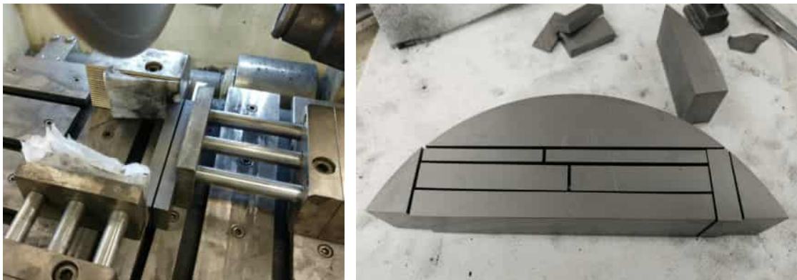
Figure 4.37: Slicing process with circular saw.
