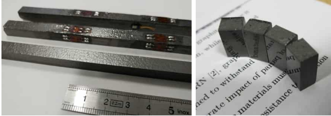
Figure 1.28: TPG samples. (Left) Samples instrumented for HRMT36 beam impact experiment ( 247 \times 7 \times 5\text{ mm} ). (Right) Polished through-plane surface, 10 mm-high samples, horizontal basal planes.
