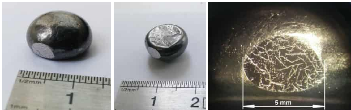
Figure 6.26: Mo-C(-Ti) LP spill material from MG-6403Fc plate. A small surface was polished to reveal its internal structure, which shows grown graphite flakes visible with optical microscopy (right).
